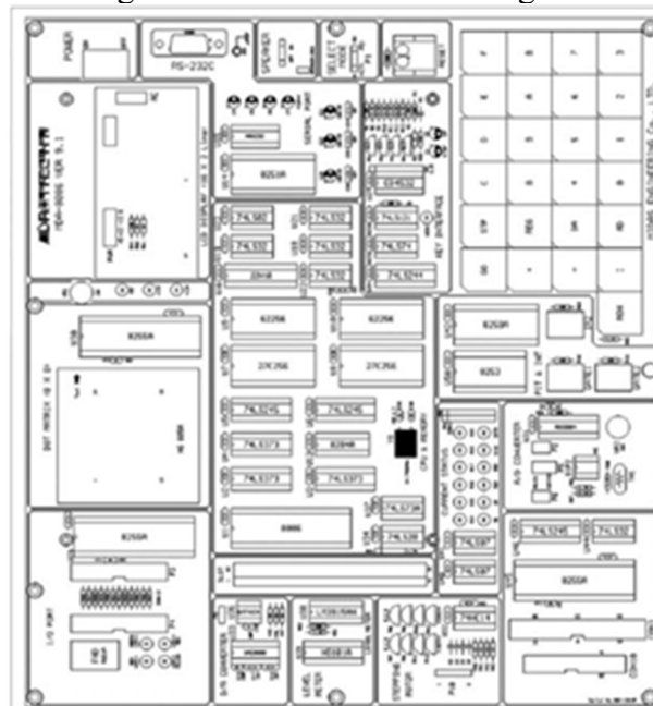
Figure 1.1: MDA-8086 Kit Diagram
