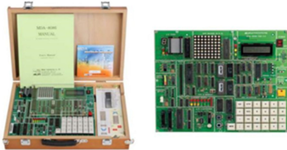
Figure 1.1: MDA-8086 Kit Diagram
